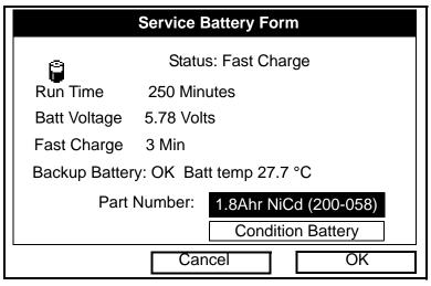
Figure 9-25: The Battery Test Option
